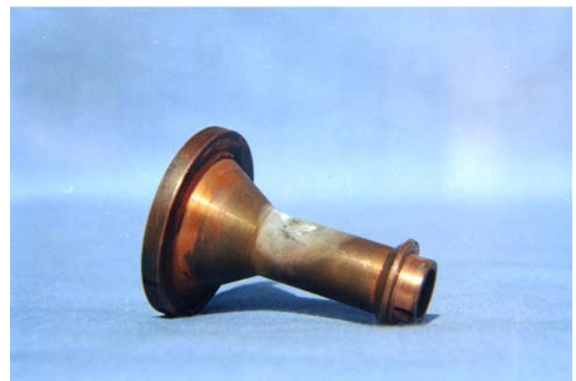
Fig. 2 Incrustation pattern at the outer surface of the arc anode (Ref 12)
